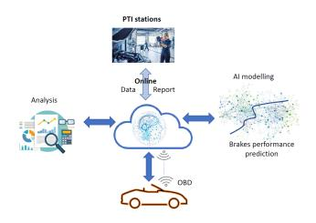
Laboratory for motor vehicles safety (University of Belgrade Faculty of Mechanical Engineering, Serbia) in cooperation with National Association of PTI stations in Serbia, supported by DEKRA Serbia, developed an advanced software for centralized real- time acquisition (online and offline), processing, and reporting on data obtained from all roller brake testers in PTI stations.
