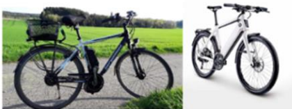
Figure 2: An EPAC (L) 3 and a type approved cycle designed to pedal in L1e-B (R) 4
