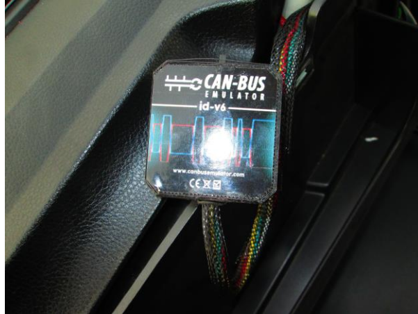
Figure 31 Urea emulator device picture used in the project
