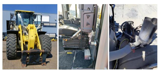
The above images show the SEMS system built into a mobile machine. The middle image shows the SEMS registration box under the seat in the cab. The right image shows the NOx sensor, the ammonia sensor and the temperature sensor (thermocouple) mounted in the exhaust of the mobile implement.
