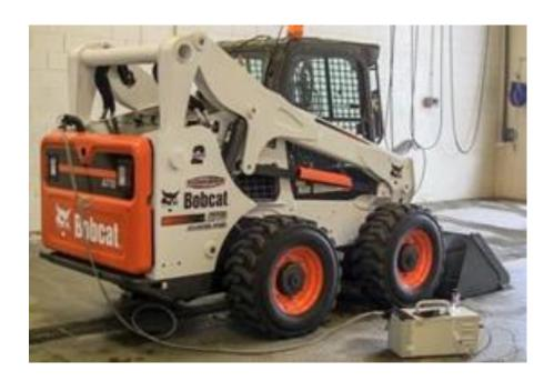
The measurement is carried out at low engine idle speed. The limit value is considered to be 250,000 soot particles per cubic centimeter. This roughly corresponds to a filter efficiency of 95%. In 2021, new types of particle counters will come onto the market that have been developed for checking particulate filters in the PTI of cars. From 1 July 2022, the new PTI test with particle counter will be introduced in the Netherlands for checking the particulate filter of diesel cars.
