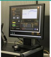
A new emission measurement that uses PN measurement instruments can assess the quality of the Diesel Particulate Filter (DPF) during the periodic technical inspection (PTI) of diesel vehicles. This was concluded after an extensive 18-month study commissioned by the Flemish, Walloon and Brussels-Capital Region in Belgium.
