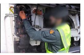
Many trucks travelling on European roads have their emission control systems disconnected, which implies a massive emission of NOx into the atmosphere. The SCR system is mandatory on Euro 5 and Euro 6 trucks. It neutralizes almost all nitrogen oxides emitted by heavy-duty trucks. However, this system can be disconnected with an "emulator".
