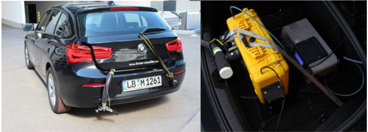
Figure 20 – Short test drive: prepared vehicle with PEMS equipment
