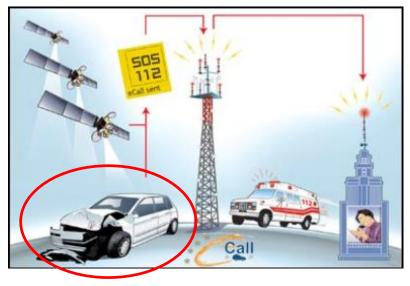
Automatically dials 112 in the event of serious accident, opens telephone link (PSAP) and communicates vehicle's location (MSD) to emergency services
