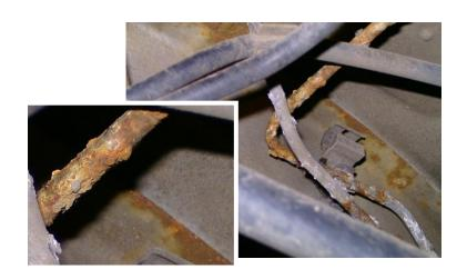
Defect → major fault break pipe - rear weak through corrosion
