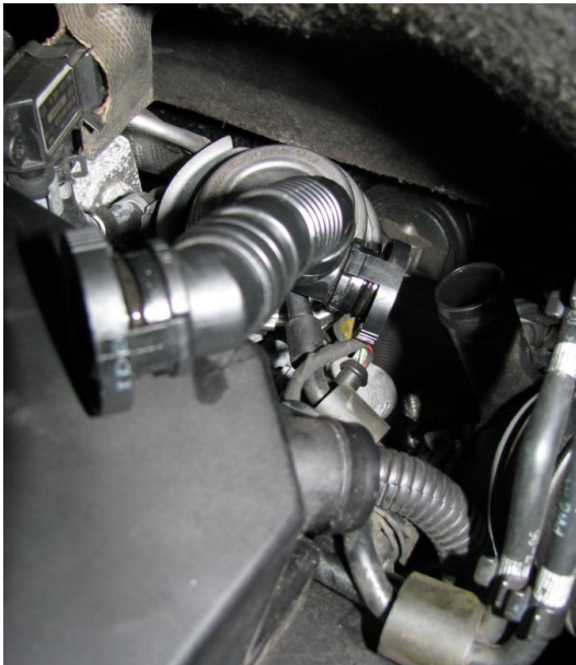
Figure 19: Vehicle 1, fault 2: Crankcase breather removed.
