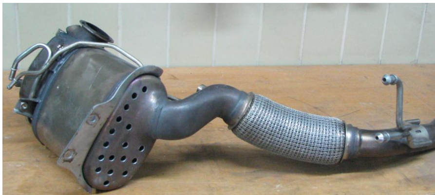
Figure 21: Vehicle 2, fault 1: DPF defect (mechanical damage).
