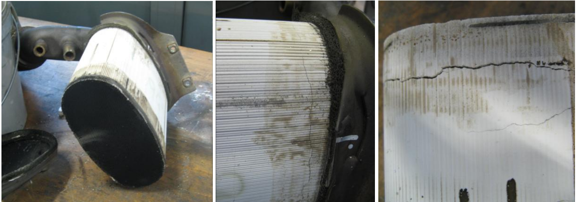
Figure 18: Vehicle 1, fault 1: DPF defect (ageing).
