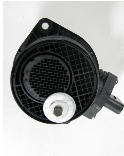
Figure 20: Vehicle 1 fault 3: manipulation of air mass flow meter.
