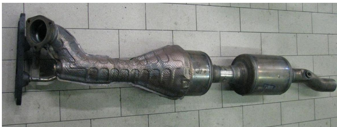
Figure 22: Vehicle 5, fault 2: ageing of SCR catalyst.
