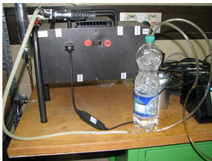
Figure 7: System used to increase the humidity of the span gas.
