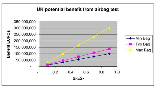
Figure 5. Overall benefit from airbag test
