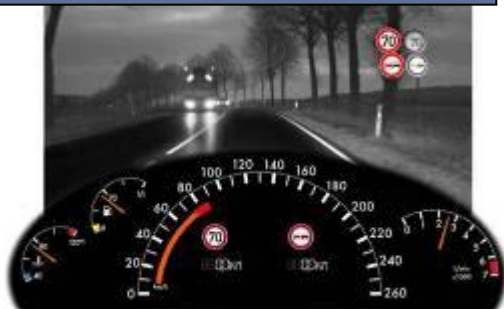
Driver's assistance by video sensing: Road sign recognition
