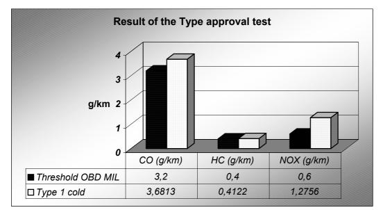
1.3.1.2 Test with combination of a altered catalyst and lambda irregularity
