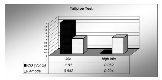
CO at low idle speed exceeds the limit value. The vehicle fails the I/M test.
