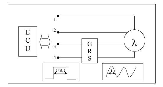
sketch: Oxygen sensor with GRS, (1 and 2 heater, 3 and 4 signal sensor
