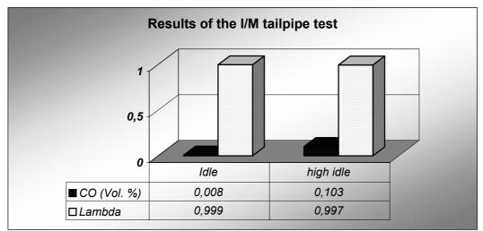
1.3.2.1 Test with a simulation of lambda sensor deterioration
