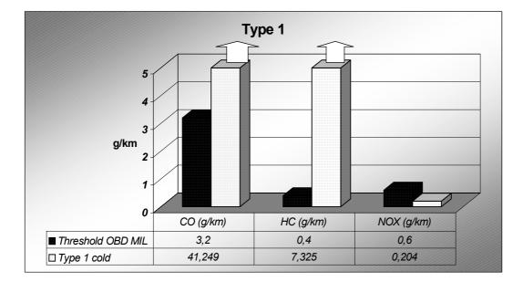
For the final type I test, the failures were MAP sensor and misfire. The throttle position did not show a relevant effect on the previous tests.
