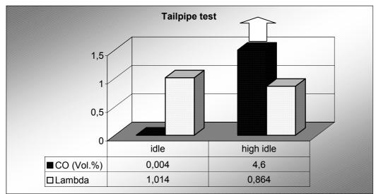
Fails I/M test. CO at high idle exceeds limit value. Lambda at high idle remain under the limit.
