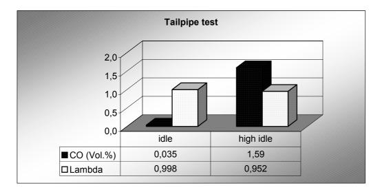
The vehicle fail the I/M test. CO at high idle exceeds the limit value.
