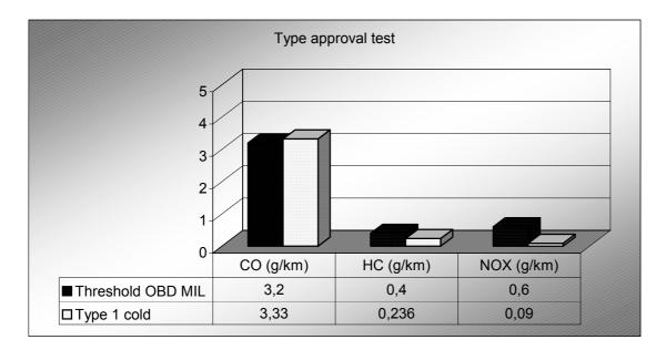
The CO result exceeds EOBD and Euro III limits. The HC result exceeds the Euro III limits.
